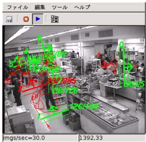
Fig. 4. Analyzing customers' action: Vitracom Siteview is used to analysis of customers' behavior. Siteview is video-based counting device. It can count objects crossing the counting line and can detect and track the objects using optimization algorithms.
